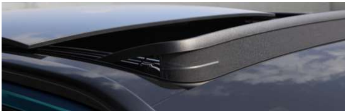
Spoiler Trapa electrica
